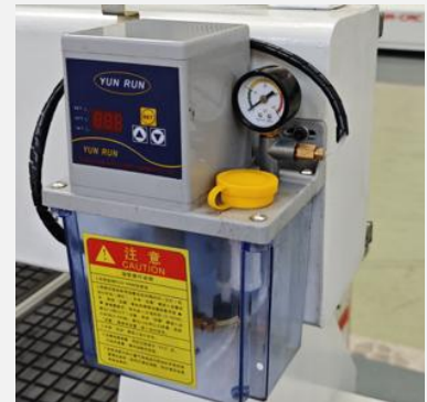
Automatic oil system
