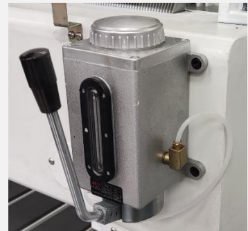
Oil lubrication system
